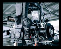
The ARRI SRH 360 is the updated ARRI SRH-3. The stabilised head can be operated by hand wheel or joystick controllers. Pan and Tilt up to 240 degrees, with the slip ring allowing unlimited rotation of the head.
