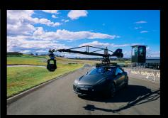
The RADICAL features 9ft, 12ft and 14ft reach with a 20kg payload capacity, producing enough torque to swing camera packages 360° in less than 6 seconds at continuous high speed. The RADICAL is versatile enough to be packed up and shipped in 6 flight cases to any location.
